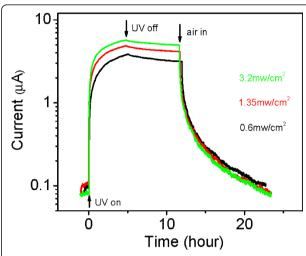
**Figure 3 Photoconductivity at three UV intensities in vacuum.** Same bias voltage and UV wavelength as in Figure 2. The steady-state currents have not been reached after about 5 h. The wire is kept in vacuum until air is let in after about 12 h (marked by a vertical arrow). The current at t=0 is higher than that in Figures 1 and 2 because the UV was turned on before the dark current had reached its minimum.
