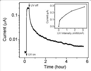
Figure 2 Transient photocurrent of the ZnO nanowire in air under UV illumination. The intensity of the  $\lambda=313$  nm light is approximately 1.3 mW/cm². Inset: steady-state photocurrent versus light intensity in air. The bias voltage is 0.3 V and is the same for all other photocurrent measurements.
