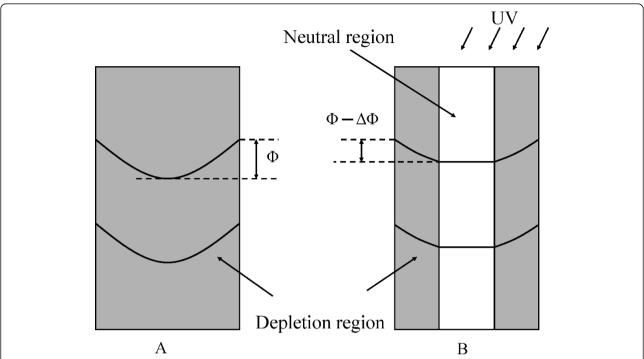
**Figure 5 Schematic of the depletion region in the dark (A) and under UV illumination (B)**. Photogenerated holes accumulate at the nanowire surface, partly neutralizing negatively charged absorbed oxygen species, which reduces the surface potential, leading to a reduction of the depletion width and increased photocurrent.
