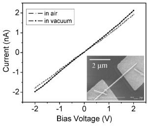
Figure 1 Dark current versus voltage of the ZnO nanowire. In air (unfilled squares) and in vacuum (filled squares). The measurement was performed after the device was kept in the dark for several days. Inset: SEM image of the device. The diameter of the wire is approximately 110 nm, and the gap between the electrodes in test is approximately 1.8  $\mu$ m.
