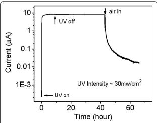
**Figure 4** Photoconductivity of the ZnO nanowire in vacuum when illuminated with multi-line UV light. Light intensity is approximately 30 mW/cm<sup>2</sup>. The bias voltage is 0.3 V.
