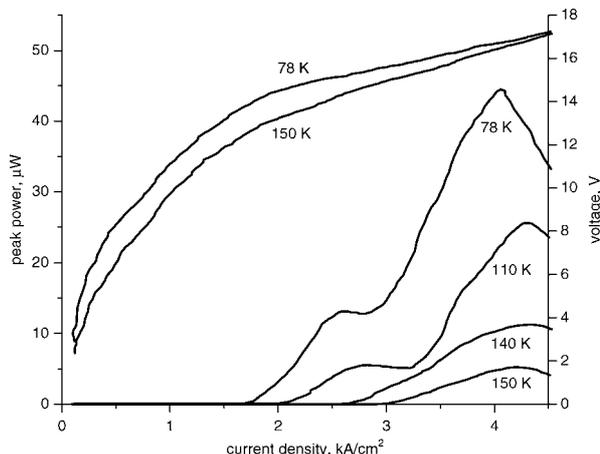
**Fig. 2** Light-current (bottom and left axes) and current-voltage (bottom and right axes) characteristics of device processed from material grown at 6 Å/s obtained at different temperatures
