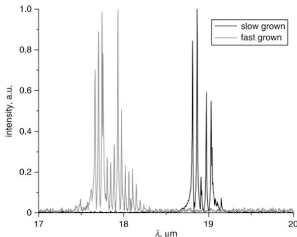
**Fig. 3** Emission spectra of slow- and fast-grown devices obtained at 80 K in pulsed mode
